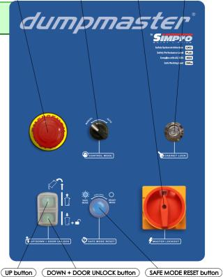
(E-STOP) (CONTROL MODEL switch) (MASTER LOCKOUT) (CABINET LOCK)
